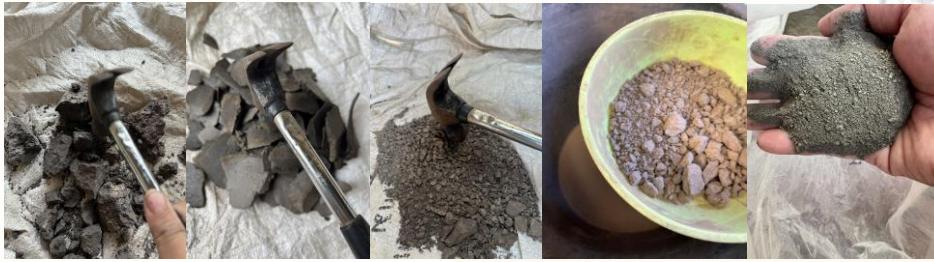
Figure 6: The clay from sample 1 and sample 2 was ground into a fine powder.
